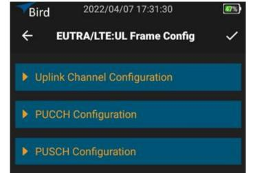
In the interface, configure the channel type of each subframe in the uplink frame. Uplink Channel Selection can choose PUCCH/PUSCH and PRACH  $_{\circ}$
