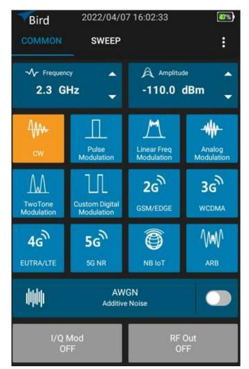
• Frequency is the carrier frequency of RF output. The settable range is 10M-6GHz, and the default is 2.3GHz. After setting the value, press OK to take effect. As shown in the picture:
