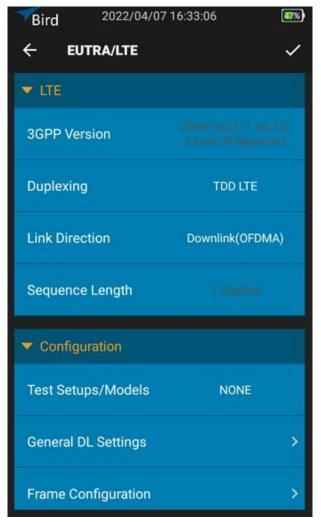
When the configuration information in the interface is completed, click " $\checkmark$ " on the top of the interface to indicate that the signal configuration is completed.
